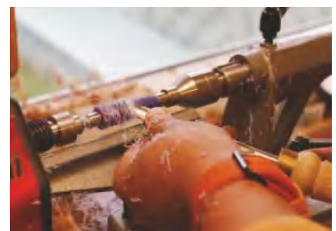
▲ Pic.6 I find it easier to work left- or right-handed to suit the direction I'm turning
